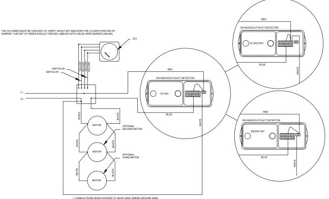
1. CONDUIT RUNS WHICH EXCEED 72" MUST HAVE GREEN GROUND WIRE. 2. FLEX CONDUIT MEETE SECURED WITH A CONDUIT CLAMP (48289) WITHIN 12" OF CONDUIT TERMINATION AT THE HANDI-BOX OR ACTUATOR. CONDUIT RUNS MUST ALSO BE SECURED ALCON GLEEVE AT A MAXIMUM OF 24" OF CONTER.
